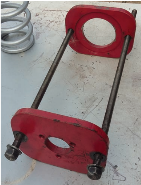
Pic 3: Safety Spring compressor
