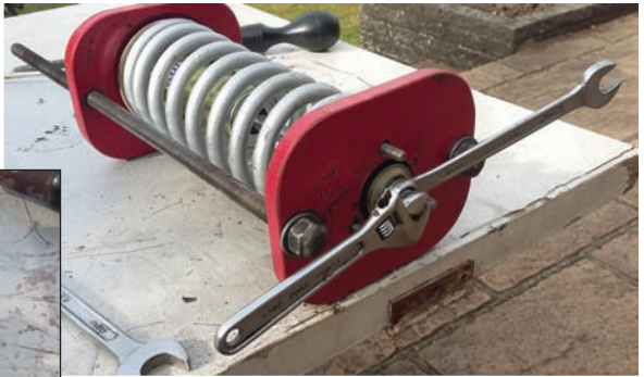
Pic 6. Tightening the locknut
