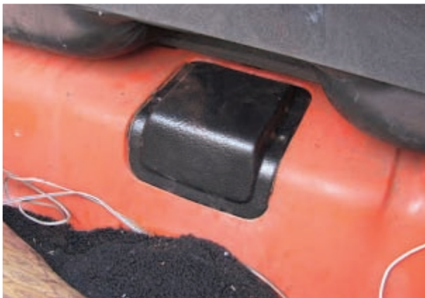
Pic1: Rarebits4classics modified spring access plate
