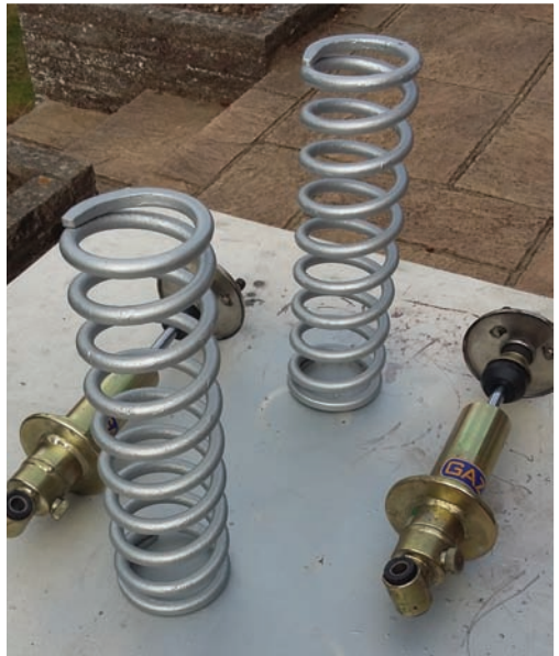
Pic 4. Gaz dampers and springs
