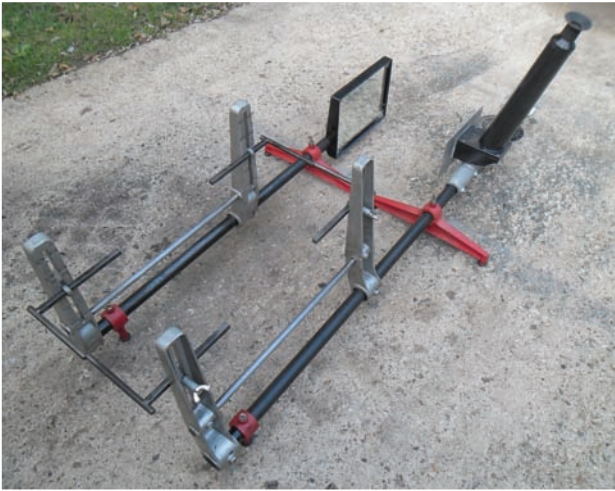
Pic 2: Optical alignment gauge
